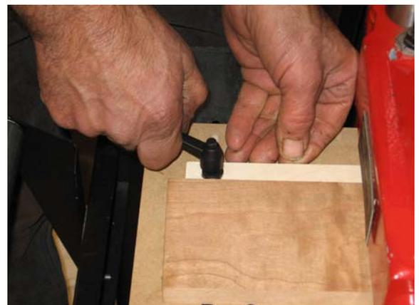
The guide locking handles have a ratchet built into them, just push down on the top button and pull up on the handle and turn it to get the handle out of your way.
