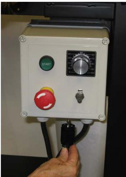
The Vari-Feed motor plugs into the center of the bottom of your control. Plug it in and twist it  $\frac{1}{4}$  of a turn to lock it in place.
