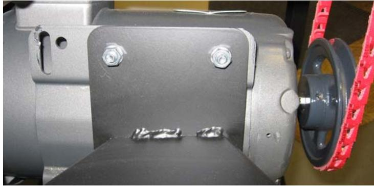
Offset the motor within the clearance of the elongated slots to find a running position that puts the motor on the same plane as the bed of the machine
