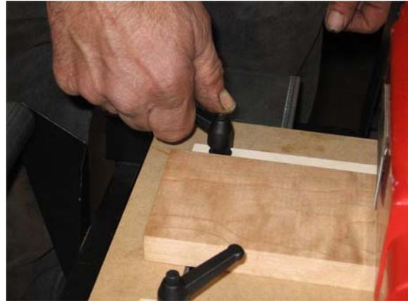
Push the flex guide adjacent to the stock and tighten one end first. Then push enough on the other end to put some flex pressure on the stock. Use a deflection pressure of 1/32" and tighten the last handle. Raise the machine head and slide a longer piece of stock in between guides to see if the guide tension is what you desire. Adjust it to suit your need.
