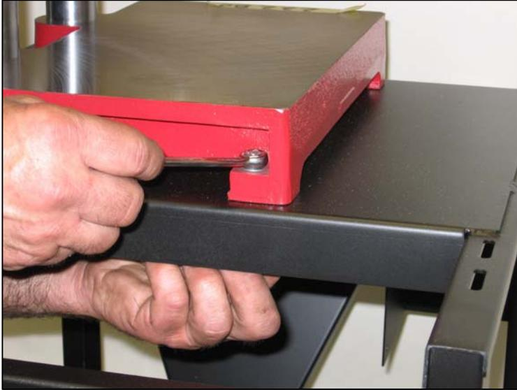
Bolt the machine base to the stand using (4)  $\frac{1}{4}$  x 1  $\frac{1}{2}$ " long hex head bolts and lock washers. *Use the nuts that held the machine to its shipping pallet.*
