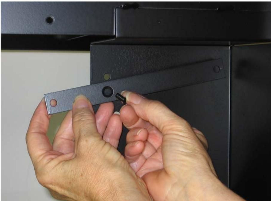
Your machine has been packed with two control mounting braces and two #10 flat head screws, lock washers and nuts. They are packed in the box under the machine head. The brace shown here is being mounted to the top of the black sheet metal control mounting enclosure. Use one of the flat head #10 screws, lock washers and nuts to mount the
