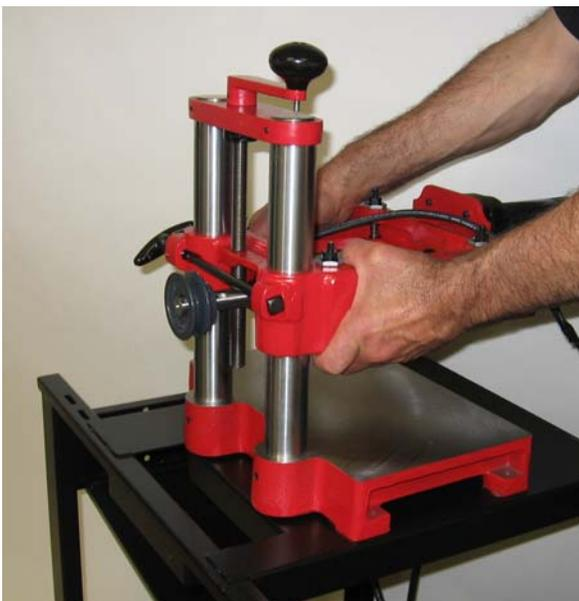
Place the machine on the stand with the pulley side of the machine over the belt cut out area in the stand.
