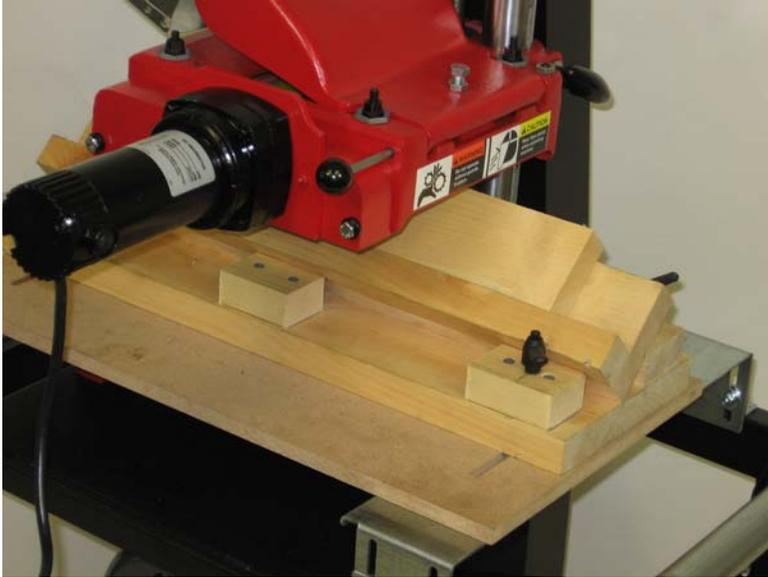
Some profiles are too deep to make on the W&H. In some cases you can rotate the profile into a flatter position to effectively reduce the depth of cut. A “**vee block**” guide would be made to guide your stock. The profile knives would have to be custom made to use in this vee block position.
