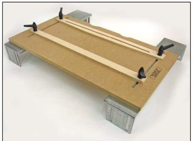
Turn the GS1 assembly upside down and mount the four angle brackets onto the bed extensions using eight of the lock nuts. **Do not tighten.**
