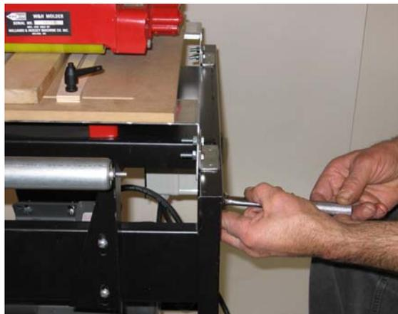
Tighten the (8) lock nuts joining the bed extensions to the angle brackets.
