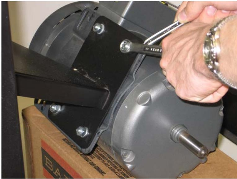
Mount the motor on the mount with (4) 5/16" x 3/4" long bolts, flat washers, lock washers and nuts. *Do not tighten yet.* The motor is mounted with the shaft end in line with the cut out for the belt in the machine mounting area.
