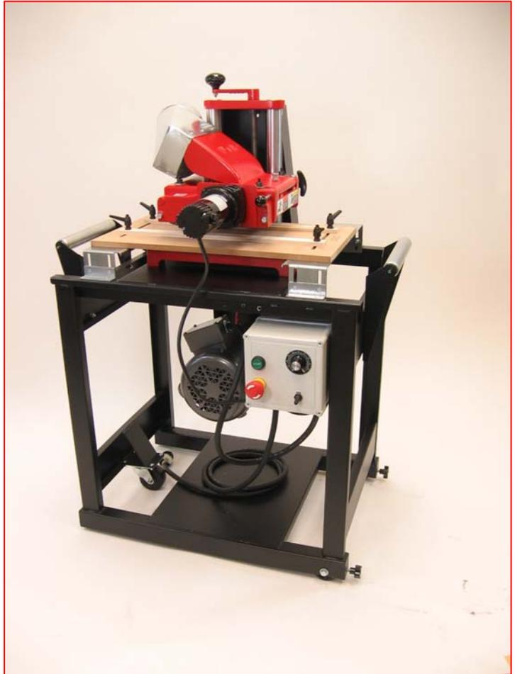
\*The crank handle will hit the chip deflector at 6.” For convenient operations at heights of over 6,” the optional crank extension 54-306 is available.
