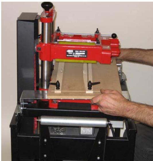
Turn the GS1 right side up. Raise the W&H molder head several inches. Insert the GS-1 assembly through the open side and over the machine bed as you guide the angle brackets into their slots in the top of the stand. Centralize the guide system relative to the length of the machine base.
