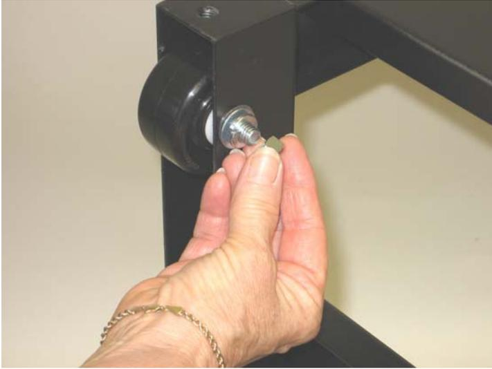
Place solid wheels in the channel of the bottom of the roller stand. Insert the 3/8" x 2 1/4" axle bolts through the holes provided.
