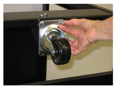
Mount castor wheel on its base with (4) 1/4"x 5/8" round head machine screws, lock washers, and nuts.
