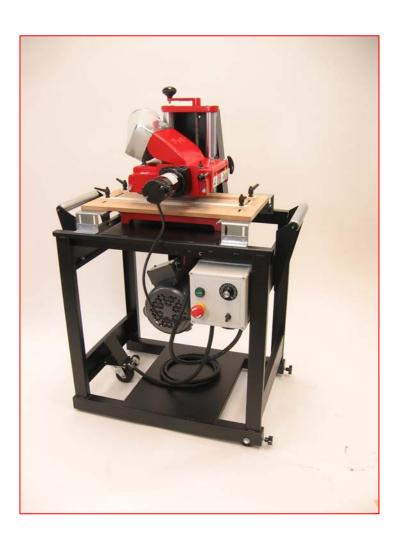
\*The crank handle will hit the chip deflector at 6." For convenient operations at heights of over 6," the optional crank extension 54-306 is available.
