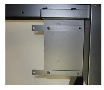
Both braces are shown here mounted to the control enclosure.
