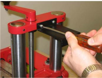
Install the belt guard bracket. Use (2) 10-24 x <sup>1</sup>/2" screws and lock washers.
