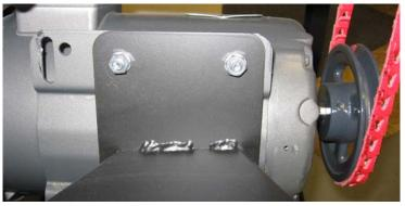
Offset the motor within the clearance of the elongated slots to find a running position that puts the motor on the same plane as the bed of the machine
