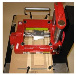
Crank the machine head down to hold your stock. Do not let the knife dig into the stock.
