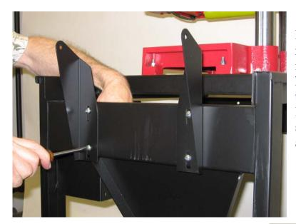
Mount the vertical roller support brackets in pairs, left and right hand on both ends of the stand. Use ¼"x 5/8" long round head screws, lock washers and nuts.
