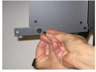
This view shows the second brace being mounted to the bottom of the control mounting enclosure. Use the one remaining #10 flat head screw, washer and nut mounted in the center hole of the bracket as you did with the first brace.
