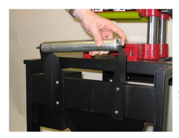
Install the two external stock rollers.
