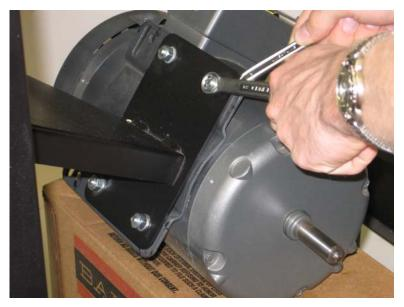
Mount the motor on the mount with (4) 5/16" x <sup>3</sup>/<sub>4</sub>" long bolts, flat washers, lock washers and nuts. *Do not tighten yet*. The motor is mounted with the shaft end in line with the cut out for the belt in the machine mounting area.
