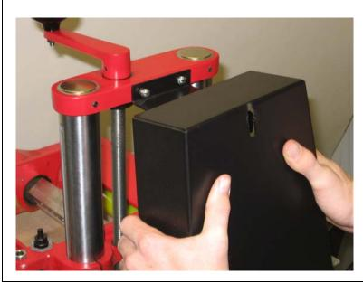
Take the belt guard and mount it over the top of the bracket and just start a  $\frac{1}{4}$ " x  $\frac{5}{8}$ " round head screw with a flat washer in threaded hole in the bracket.
