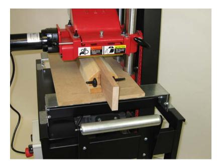
When **planing the edge** of stock, a high, square, relieved guide is needed in order to have the edge reasonably square and to provide stability. The center reliefs are to reduce friction.
