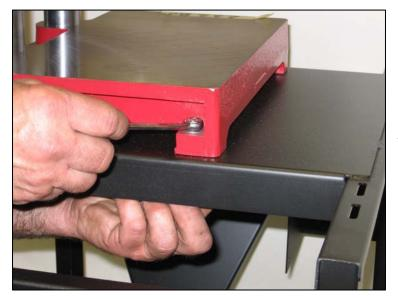
Bolt the machine base to the stand using (4)  $\frac{1}{4} \ge 1 \frac{1}{2}$ " long hex head bolts and lock washers. Use the nuts that held the machine to its shipping pallet.
