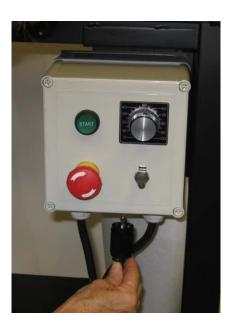
The Vari-Feed motor plugs into the center of the bottom of your control. Plug it in and twist it <sup>1</sup>/<sub>4</sub> of a turn to lock it in place.
