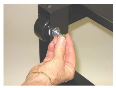
Place solid wheels in the channel of the bottom of the roller stand. Insert the 3/8"x 2  $\frac{1}{4}$ " axle bolts through the holes provided.
