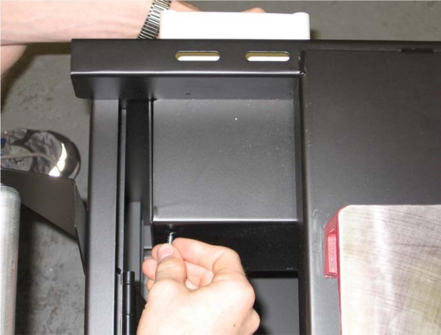
To mount the switch, align the (4) holes in the back of the switch box to the (4) in the stand mounting box. Partially start all four screws then tighten them evenly. ***Be careful not to over tighten the screws.***
