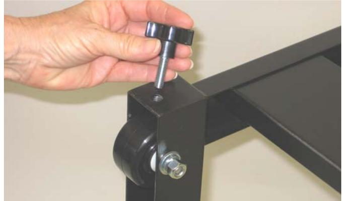
Install brake knobs in threaded insert on end of the stand.
