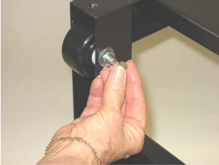
Install the flat washer, lock washer, nut and tighten.
