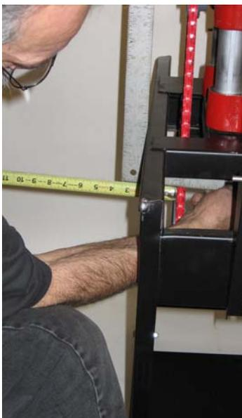
Align the belt so that the belt travels in a straight line from one pulley to the other.
