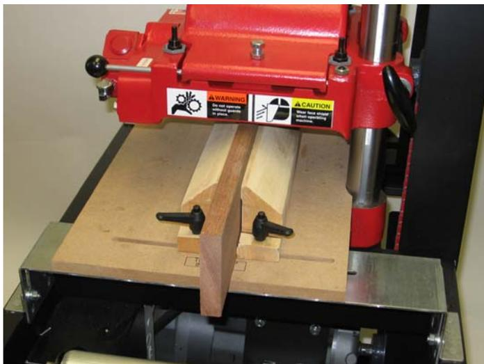
When **planing the edge** of stock, a high, square, relieved guide is needed in order to have the edge reasonably square and to provide stability. The center reliefs are to reduce friction.
