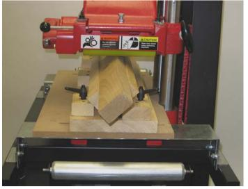
When making **tongue and groove stock**, a serious and detailed approach is needed in order to achieve a uniform fit. Carefully pre-inspect your stock for cupping and warping. You need to plane all your stock to one uniform size.
