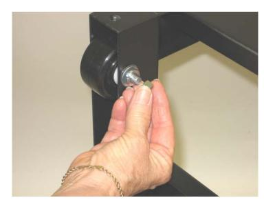
Install brake knobs in threaded insert on end of the stand.
