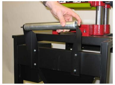
Install the two external stock rollers.
