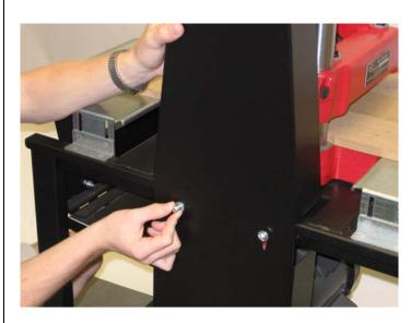
Lift the guard slightly and start the (2) lower ¼"x 5/8" round head screws with flat washers. Tighten all three guard screws
