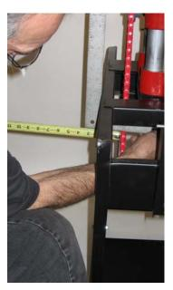
Align the belt so that the belt travels in a straight line from one pulley to the other.
