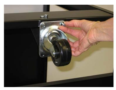
Mount castor wheel on its base with (4) 1/4"x 5/8" round head machine screws, lock washers, and nuts.
