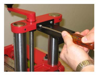
Install the belt guard bracket. Use (2) 10-24 x ½" screws and lock washers.
