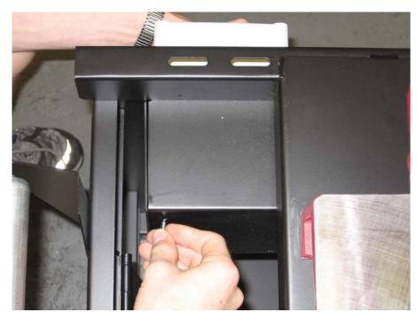
To mount the switch, align the (4) holes in the back of the switch box to the (4) in the stand mounting box. Partially start all four screws then tighten them evenly. Be careful not to over tighten the screws.
