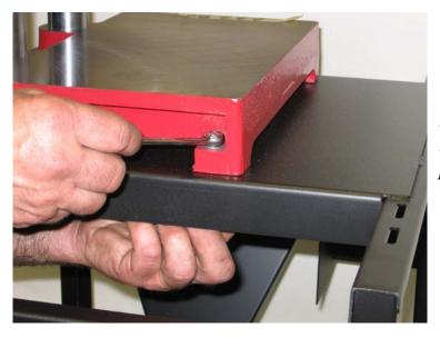
Bolt the machine base to the stand using (4) ½ x 1 ½" long hex head bolts and lock washers. *Use the nuts that held the machine to its shipping pallet.*
