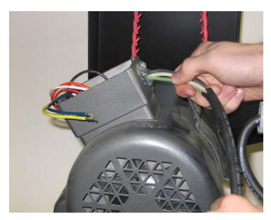
Install the cord connector to the motor and insert the cord so that the casing is clamped in the connector. Now follow the wiring instructions.
