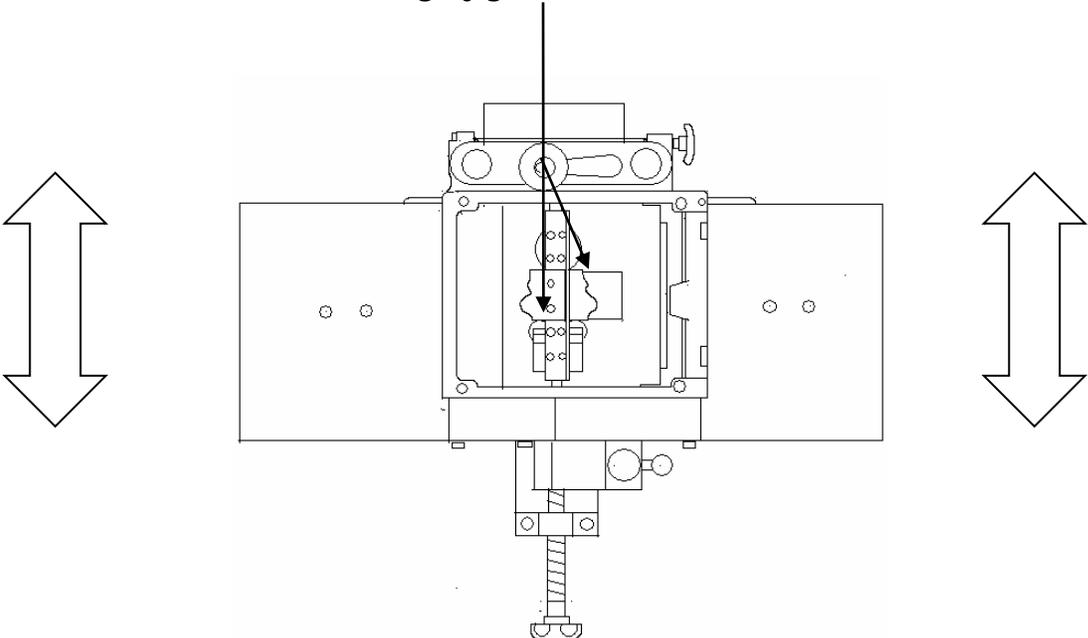
Now that your jig is aligned you will need to secure it to the machine bed or extended beds if you have them. The extended bed is part of our older guide system. If you have the newer GS-2 guide system, replace it with the elliptical jig.
