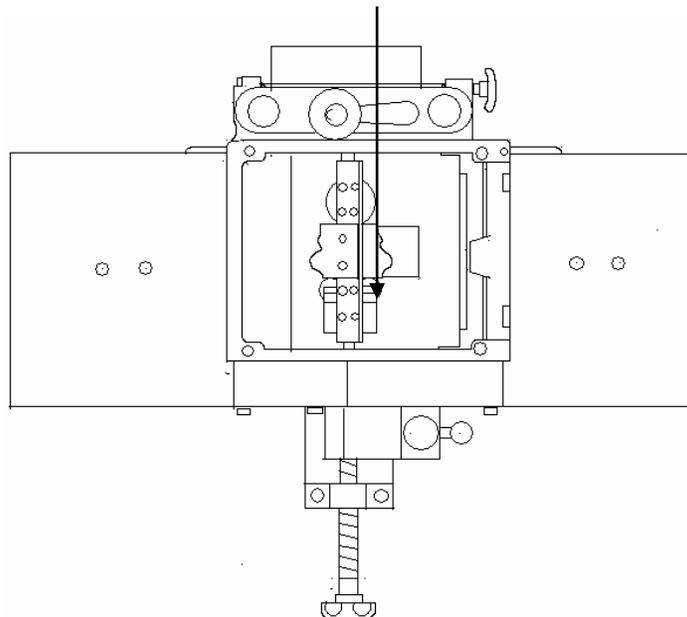
Position the jig so the fixed bearing aligns with the center of the machine arbor and stock aligns with knife profile. (See Illustrations 4 & 5). **NOTE** The fixed bearing has two positions. The outer position is used for wider moldings.
