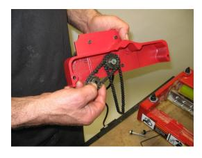
Some chains may have master links. Install the chain with the rounded end of the master link clip moving in the direction of chain travel.
