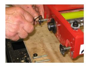
Pick up the vari-feed unit and put the new **54 pitch long chain (outfeed roller chain)** over the driving sprocket closest to the chain guard housing. Put the **new 36 pitch short chain (infeed roller chain)** over the outer driving sprocket
