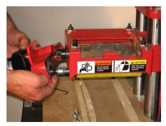
Pivot the infeed swing arm up in position and reinstall the rest screw (54-16) with thread locker, then reinstall the pressure screws, pressure screw guides, and springs.
