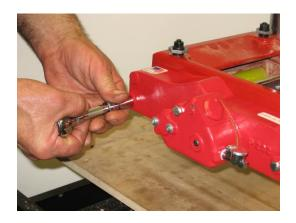
Remove both P-111 (15 tooth) axle sprockets, replacing them with the VF-3 (14 tooth) sprockets (hub first), using thread locker on the setscrews setting the outfeed sprocket 5/32" in from the end of the axle and the infeed 1/16" in from the end of the axle.
