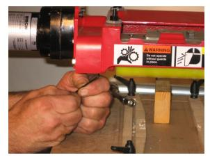
Test the **direction of travel of the feed rollers**. As you face the butt end of the feed motor the rollers should be turning in a clockwise direction.
