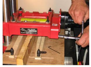
may have to make a custom adjustment using the attaching bolt hole clearance to obtain an optimum chain tension/slack setting.
