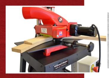
Our EJ-92 Elliptical Jig Accessory is available for moldings with a changing radius design. Customer supplied ELLIPTICAL segmented material attaches to a matching template. The fixed and floating bearings run alongside the template piece following the shape of the molding.
