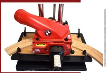
All models will also mold CONSTANT RADIUS moldings! Customer supplied radius guides, matching radius segmented material and a set of W&H profile molding knives and you're good to go! Switch from molding radius pieces to straight pieces just by switching out the guides.
