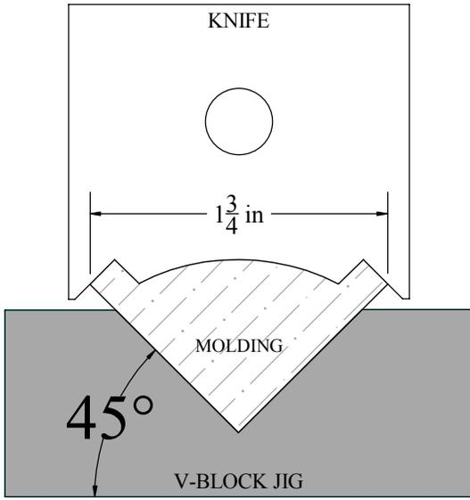
Due to a depth of cut greater than 3/4" this knife will need to be used in conjunction with a customer supplied V-block, typically made of wood.
