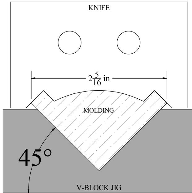
Due to a depth of cut greater than  $\frac{3}{4}$ " this knife will need to be used in conjunction with a customer supplied V-block, typically made of wood.
