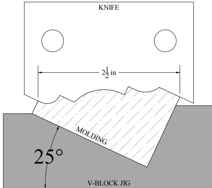
Due to a depth of cut greater than 3/4" this knife will need to be used in conjunction with a customer supplied V-block, typically made of wood.
