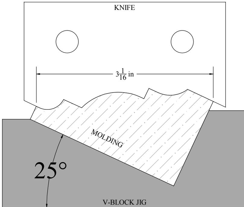
Due to a depth of cut greater than 3/4" this knife will need to be used in conjunction with a customer supplied V-block, typically made of wood.
