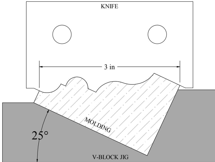
Due to a depth of cut greater than 3/4" this knife will need to be used in conjunction with a customer supplied V-block, typically made of wood.
