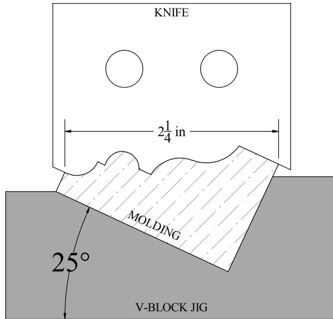
Due to a depth of cut greater than  $\frac{3}{4}$ " this knife will need to be used in conjunction with a customer supplied V-block, typically made of wood.
