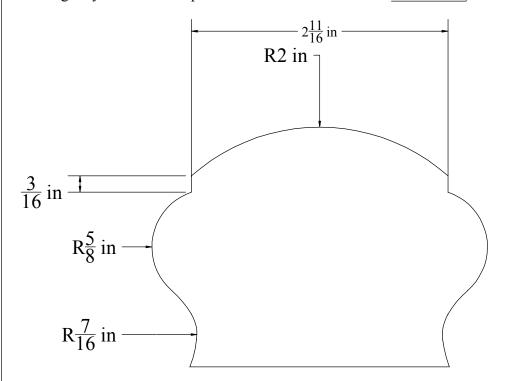
When molding handrails, multiple steps are required.
