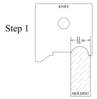
Some picture molds require an undercut, as seen in Step 1. Use taller guides to support the stock to ensure that you can support the piece properly, without trying to balance the stock on the small flat. Run the face of the mold as seen in Step 2 to complete your molding. This way, even with the undercut, the stock has a large flat on the bottom for support while molding.
