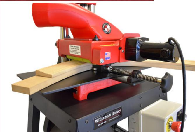
Our EJ-92 Elliptical Jig Accessory is available for moldings with a changing radius design. Customer supplied ELLIPTICAL segmented material attaches to a matching template. The fixed and floating bearings run alongside the template piece following the shape of the molding.
