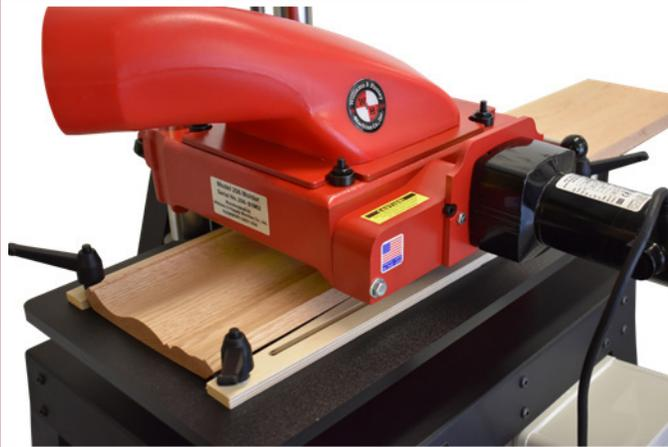
Choose from any model for Quick & Easy Set Up for STRAIGHT molding from 1/4" up to 6 3/4" wide profiles! Take advantage of the open-ended design for wide boards such as cabinet doors, raised panels, baseboards and doors.
